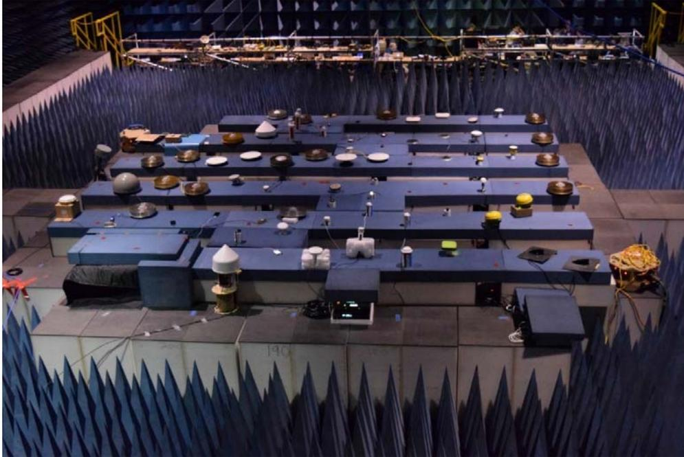
**Figure 2. GPS/GNSS Receivers in WSMR Semi-Anechoic Chamber<sup>32</sup>**
