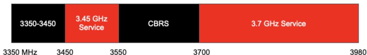
Figure 1: Inconsistent spectrum uses in the U.S. 3 GHz band that could result from failing to consider 3.35-3.45 GHz incumbent operations when adopting rules for 3.45-3.55 GHz
