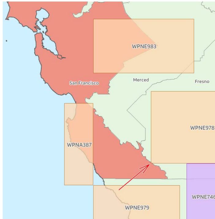
Figure 2 - An RSA in the Fresno, CA PEA overlaps into the San Francisco, CA PEA, slightly impairing an additional channel
