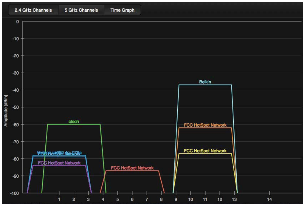
Figure 4 - InSSIDer RF channel measurement during CableLabs test
