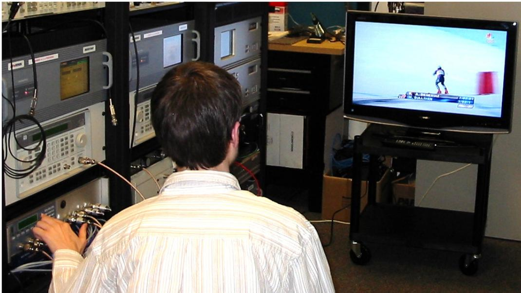
A very high interfering signal powers it was noticed that some receivers had difficulty tuning in to Channel 6, although they would deliver an unimpaired picture if they were receiving before the interference was raised. Consequently, tests were performed at every interference
