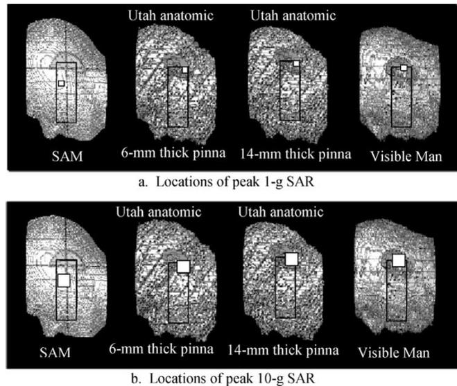
Fig. 6. Locations of the peak 1- and 10-g SAR regions (shown as white squares) for the SAM model and for three anatomical models for the “cheek” placement of the handset using a 20-mm-long helix antenna at 835 MHz. Whereas the peak 1- and 10-g SAR regions for the anatomic models include the lossy pinna, the highest SAR regions for the SAM model similar to [7] and [8] are considerably lower (by approximately 2.5 cm) in the cheek region.
