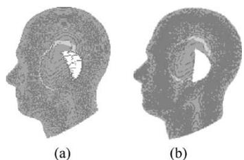
Fig. 3. (a) Original plastic-ear SAM. (b) Proposed lossy-ear SAM. In addition to using lossy tissue-simulant dielectric properties, the "ear" is rotated by  $24^\circ$  to have a more natural appearance of the "ear" vis à vis the cheek.
