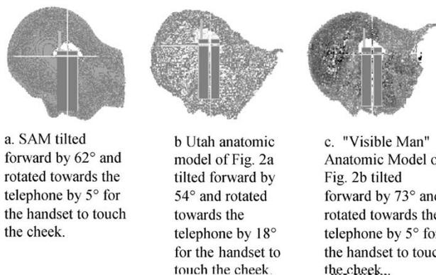
Fig. 5. Tilted SAM and anatomic models used for SAR calculations for the "cheek" position with vertically placed telephones. As recommended in [3], the acoustic output point of the telephone is placed against the ERP of the SAM model (see Fig. 1).
