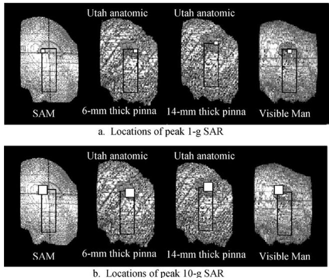
Fig. 7. Locations of the peak 1- and 10-g SAR regions (shown as white squares) for the SAM model and for three anatomical models for the “cheek” placement of the handset using a 40-mm-long monopole antenna at 1900 MHz.
