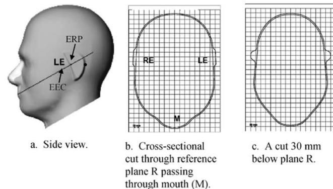
Fig. 1. SAM head model with three cross-sectional cuts defining the 5–10-mm thickness of the plastic shell for different cross sectional planes [3]. Also shown are the entrance to ear canal (EEC) and the ERPs. Rather than the EEC, the ERP is recommended by the standard for placement of the acoustic output of the handset against the SAM.
