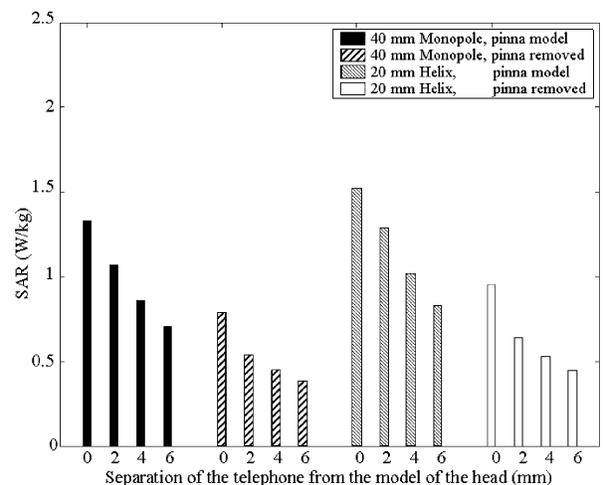
b. 10-g SAR, Utah Model, 15°-tilted position, frequency = 1900 MHz, radiated power = 125 mW.
