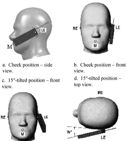
Fig. 4. Placement of a radiating handset for cheek and  $15^\circ$ -tilted positions relative to plastic-ear SAM [3].
