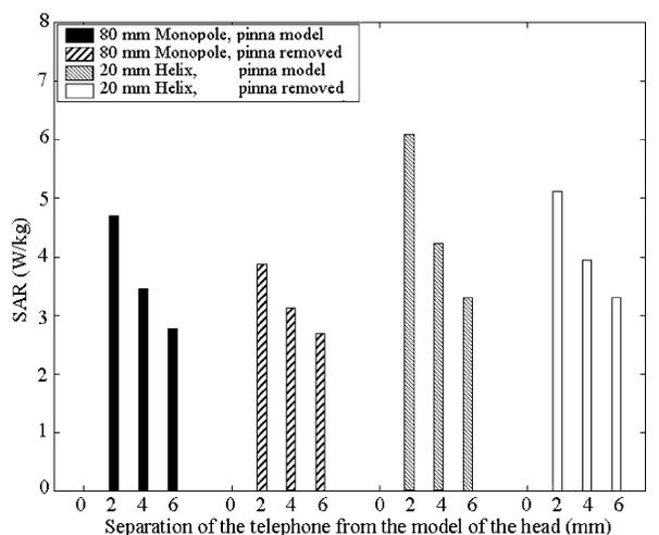
c. 1-g SAR, Utah Model, 15°-tilted position, frequency = 835 MHz, radiated power = 600 mW
