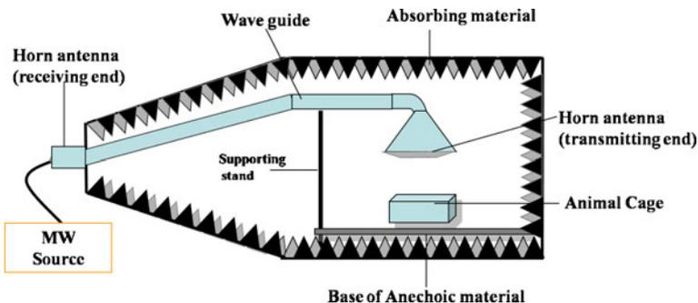
**Fig. 1** Schematic layout of 2.45 GHz exposure setup
