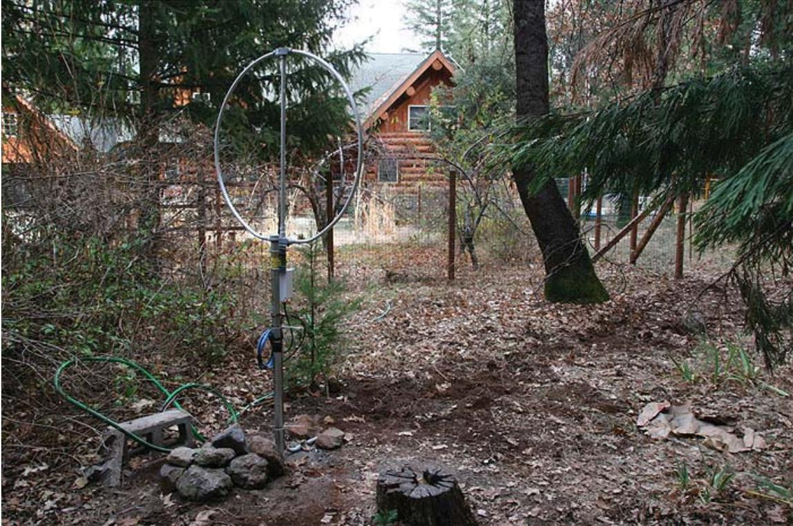
Figure 1 – Outdoor Antenna Required for Residential AM Radio Reception
